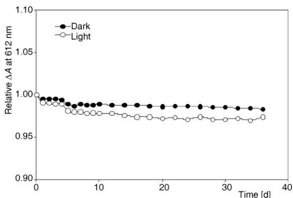
**Figure 7. Post-irradiation stability of (VBB films) stored under different storage conditions**
