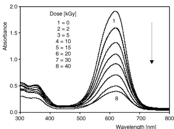
Figure 1. The absorption spectra of un-irradiated and irradiated VBB film, according to different absorbed doses; VBB = 0.5 phr,  $\lambda_{\text{max}} = 612 \text{ nm}$
