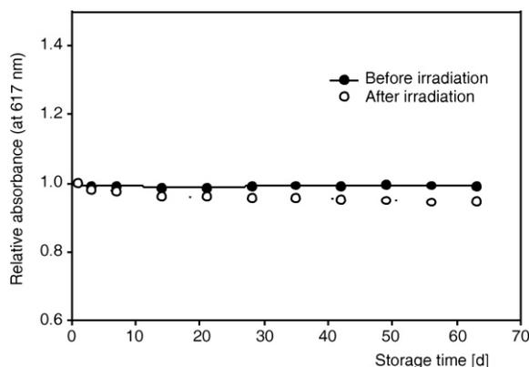
**Figure 8. Post-irradiation stability of VBB solutions [TR] =  $4.1 \times 10^{-4} \mu\text{molL}^{-1}$  and [CH] = 66.6 phr stored in direct and indirect light at room temperature, as a function of storage time, at 100 Gy**
