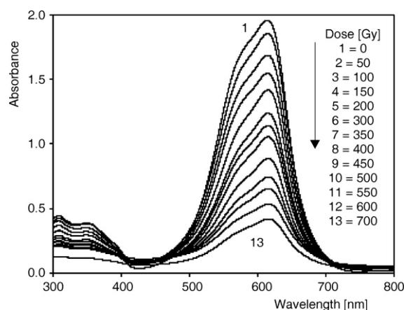
Figure 2. The absorption spectra of the un-irradiated and gamma irradiated VBB liquid, according to different absorbed doses; VBB =  $5.1 \cdot 10^{-4}$  mol L<sup>-1</sup>,  $\lambda_{\text{max}} = 617 \text{ nm}$
