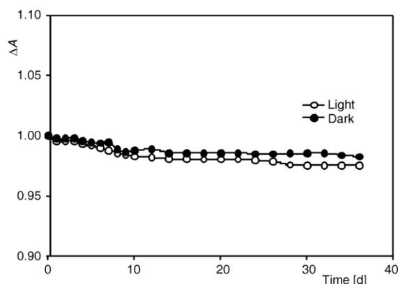
**Figure 6. Pre-irradiation stability of (VBB film) stored under different storage conditions**
