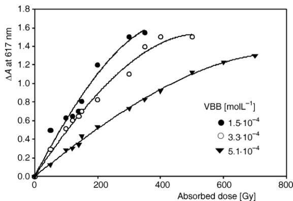
Figure 4. Dose response of the (VBB-liquid) at 617 nm in the full dose range of 0-700 Gy.  $\Delta A = A_0 - A_i$ , where  $A_0$  and  $A_i$  are absorbances of the irradiated and un-irradiated samples, respectively
