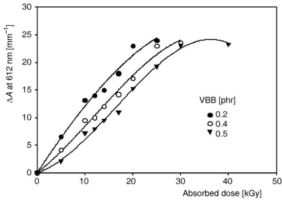
Figure 3. Change of  $\Delta A$  as a function of absorbed dose for different VBB concentrations in PVA films
