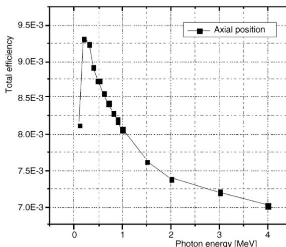
**Figure 3.** The calculated axial total efficiency of the spherical detector at a distance 10 cm from the detector surface as a function of the photon energy from 0.1 up to 4 MeV
