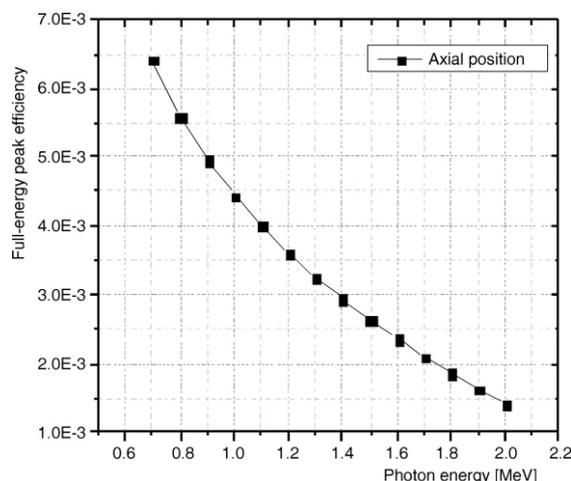
**Figure 4.** The calculated axial full-energy peak efficiency of the spherical detector at a distance 10 cm from the detector surface as a function of the photon energy from 0.7 up to 2 MeV
