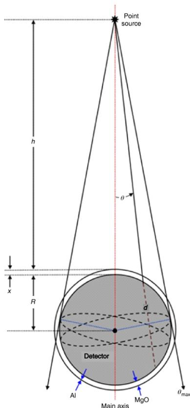
Figure 1. The point source is situated on the spherical detector main axis
