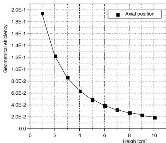
**Figure 2.** The calculated axial geometrical efficiency of the spherical detector as a function of the source-to-detector distance  $h$ , from 1 up to 10 cm
