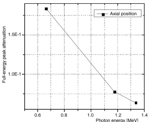
Figure 7. The calculated full-energy peak attenuation of the spherical detector at a distance 10 cm from the detector surface as a function of the photon energy
