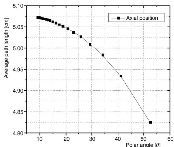
Figure 6. The average path length of gamma photon in the spherical detector as a function of the polar angle
