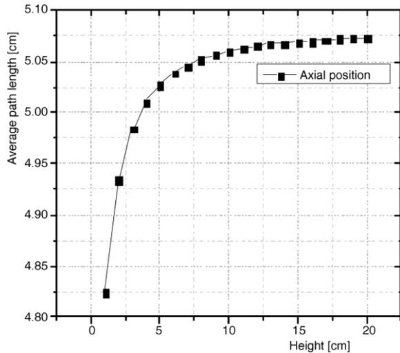
**Figure 5. The average path length as a function of the axial source-to-detector distance  $h$  from 1 up to 20 cm**
